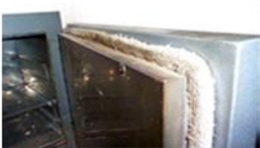
Asbestos rope seal on drying oven
